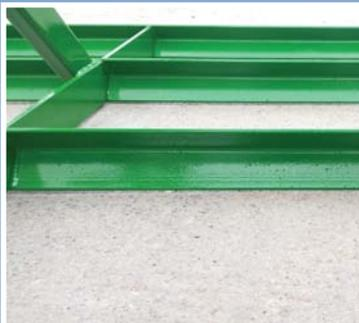
**2. Three levelling blades ensure a firm and level seed bed.**
